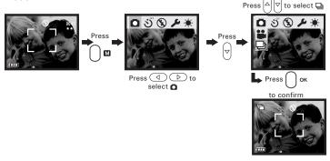
When the above setting is done, icon The appears on the LCD screen, hold down the Shutter button to record continuous pictures. You can capture 4 continues pictures each time.
